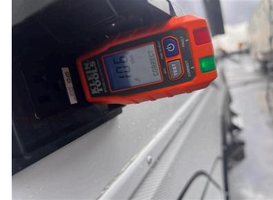
Exterior Curbside Outlet Voltage Test
